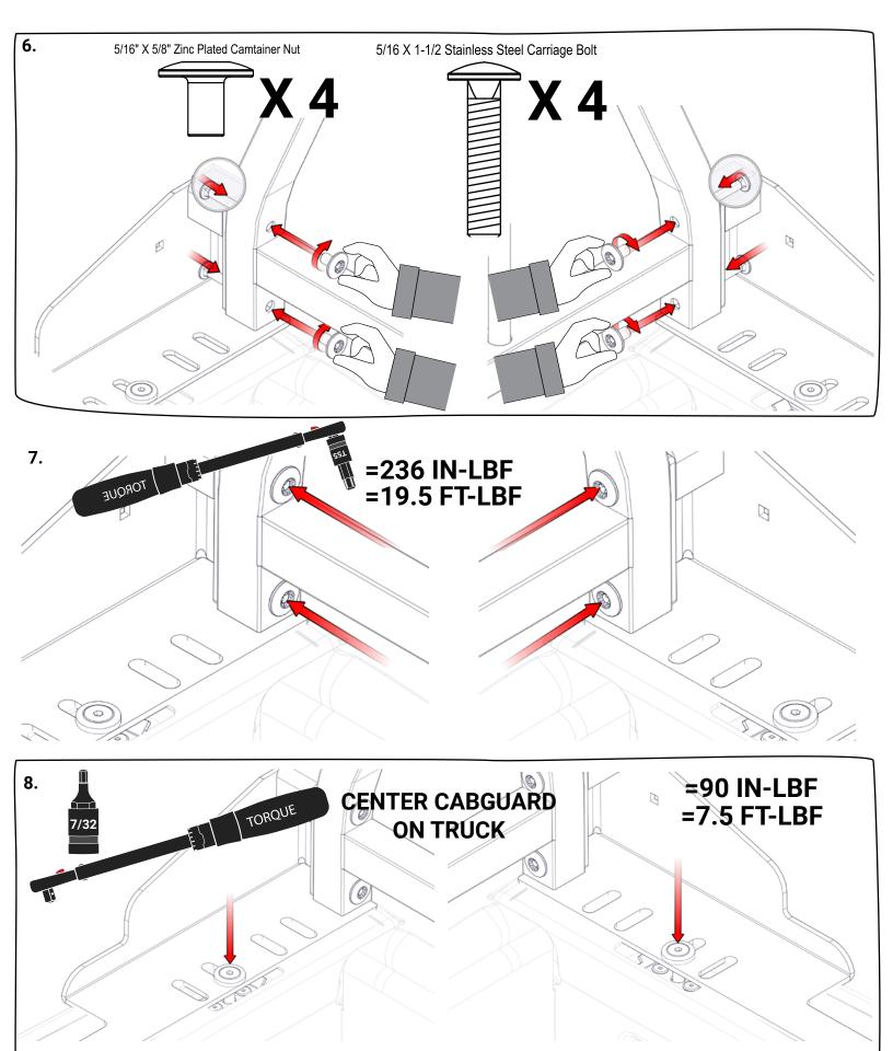
THIS STEP IS FOR INSTALLATIONS WITHOUT WESTCAN RAILCAPS ONLY. SKIP TO STEP 9 FOR INSTALLATIONS WITH WESTCAN RAILCAPS OR PROCEED TO STEP 11.
