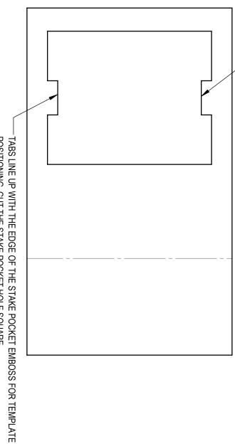
POSITIONING. CUT THE STAKE POCKET HOLE SQUARE.
