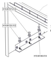
5. Place the assembly into the vehicle and secure to the floor with the H10-B133-312, ¼" x 1-1/4" full thread bolt, H10-B157-014, ¼" lock washer and H10-B146-014, ¼" washer. Apply thread lock and Torque bolts to 25 ft-lb.
