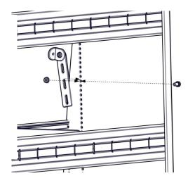
7. Mark drill locations for insert nuts and remove the bracket assembly. Install insert nuts using the method described above and replace the bracket assembly. Securely fasten the assembly to the end panel. Secure to the wall using the H10-B133-312, H10-B157-014 and H10-B146-014. Apply thread lock and torque to recommended setting as per your wall substrate. Inspect assembly to ensure all components are correctly installed.
