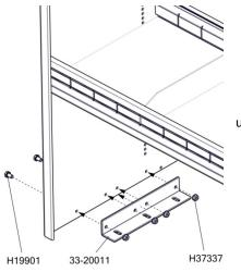
1. Fasten a 33-20011, 10" long end panel mounting bracket to each end panel. Secure using H19901, ¼" x ½" plated steel flange bolts and H37337, ¼" flange nuts.
